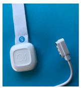
Figure 19: Gabi Band and its charging cable
