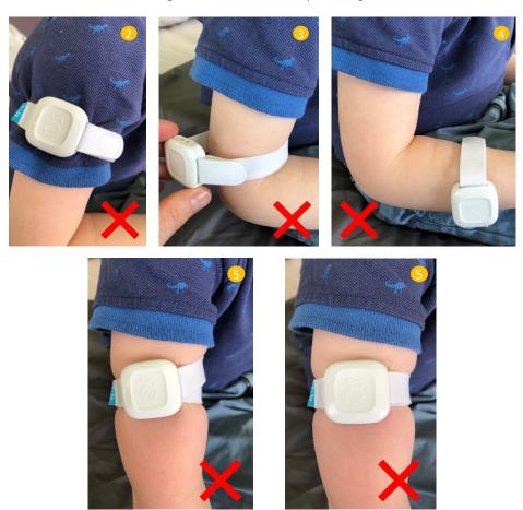
Figure 41: Gabi Band wrong positionings
