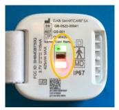
Figure 37: Green and red lights at the bottom of the sensor
