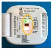
Figure 20: Green and red LEDs blinking
