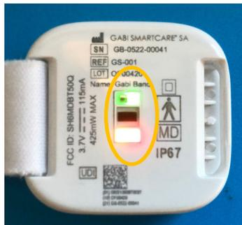
Figure 20: Green and red LEDs blinking
