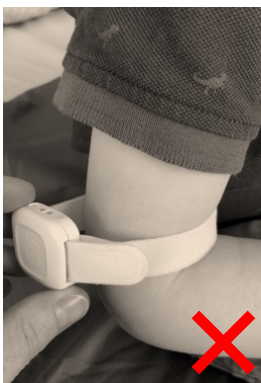
Figure 30: Bad tightening: not enough
