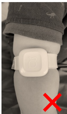
Figure 31: Bad tightening: too tight
